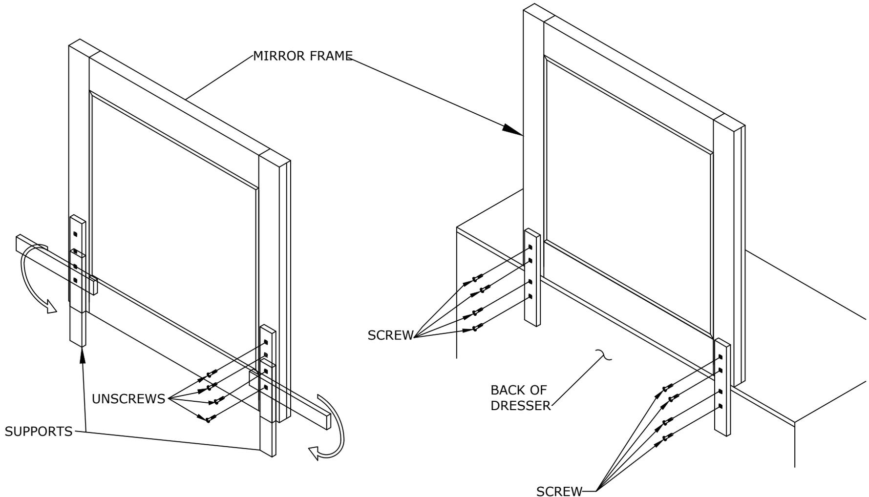
① UNSCREW FROM BOTTOM AND TOP OF THE SUPPORT LEAVING THE BOLT IN THE CENTER LOOSEN
