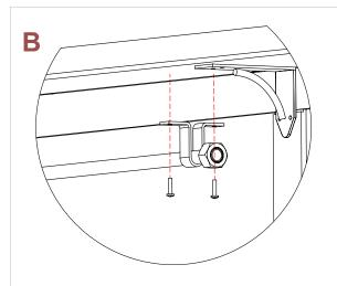
TO INSTALL THE TOWEL RAIL FIRST YOU SHOULD TO REMOVE, THIS IN THE UNDER COVER, WITH THE ASSISTANCE OF THE SCREWDRIVER REMOVE THE SCREWS. AS SHOWN IN PICTURE B
