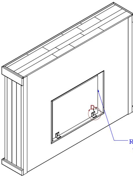
REMEMBER TO HAVE CENTERED THE CHIMNEY BEFORE FIXING IT WITH THE CABINET.
